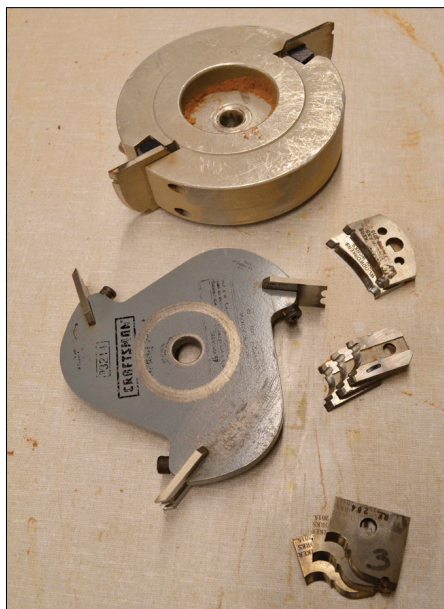
● For profiles more complex than what can be made with the table saw and planer, I use moulding heads on the table saw.
