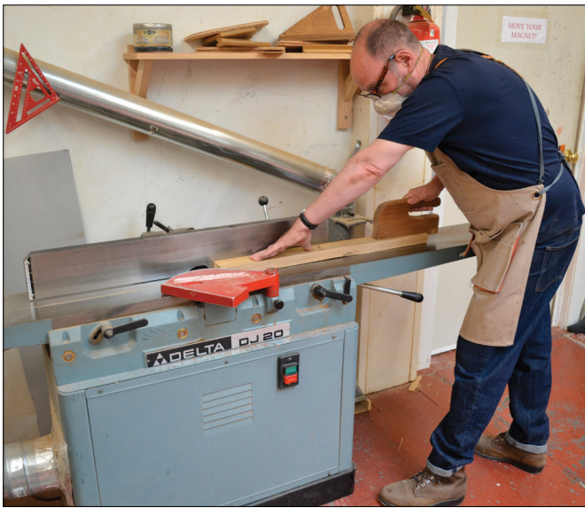
● Once I've roughed out my sides, I bring in the jointer and planer to mill my sticks flat, straight, square, and to final thickness and width.
