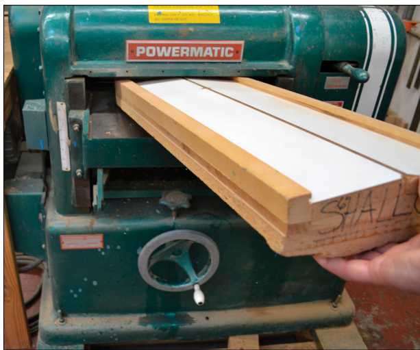
● Slopes, or bevels, can be made with a planer equipped with a sloping jig—a beveled board laid in the bed of the planer.
