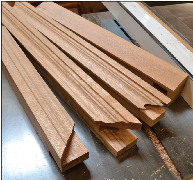
● Parts for a rain sill frame modeled after Northern Renaissance master cabinetmaker's frames.
